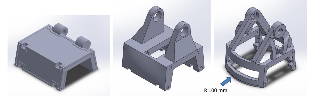
The final design was inspired by the generative design results. The large radius gives the parallel rods space to move. It was made with a guide curve in a loft.
