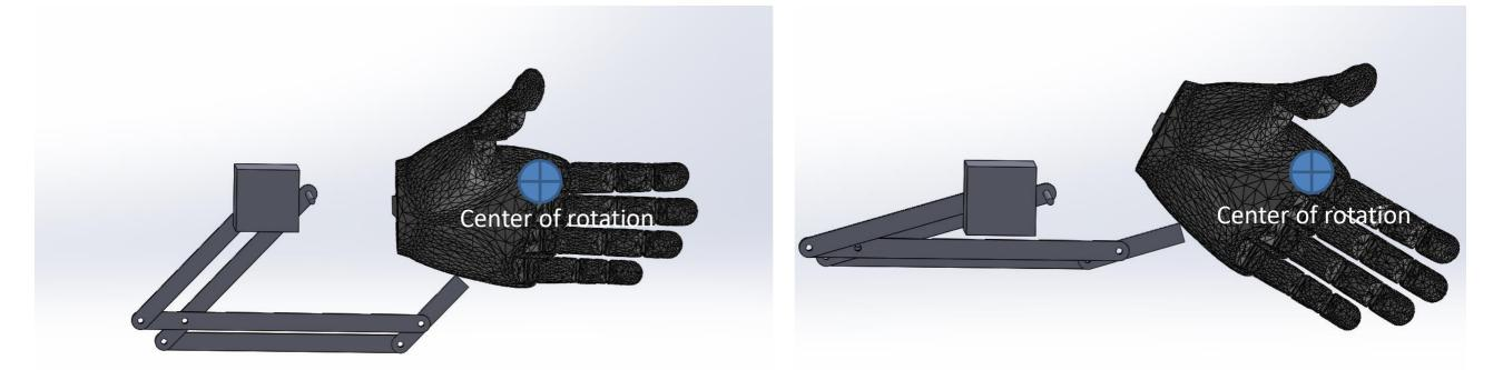
This mechanism shifts the center of rotation to the center of the hand. This was intended to pour smoothly out of a wine glass. But it's big and complicated.
