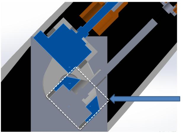
The original design bumps into the top stepper bracket when the arm is raised. Huge chamfers were added before printing.
