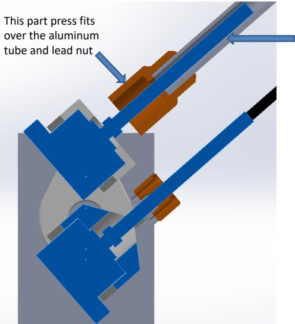
The linear stepper motor's screw is inside the aluminum tube.
